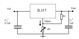
$\ast$  = Cin is required if regulator is located an appreciable distance from power supply filter.
